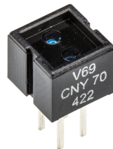
Fig. 13: Sensor CNY70 Datasheet CNY70
