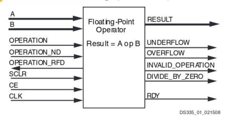
Figure 1: Block Diagram of Generic Floating-Point Binary Operator Core
